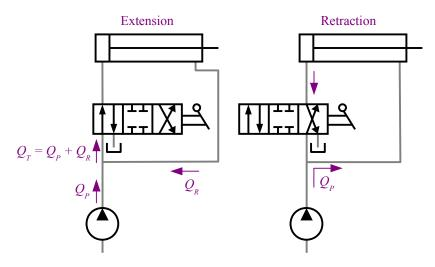
Consider a free-body diagram of the piston during extension. The pressure on both sides of the piston is the same, so the force is the pressure times  $A_1$  minus the pressure times  $A_2$ .  $F_{ext} = p A_1 - p A_2 = p(A_1 - A_2) = p A_{rod}$ . The extension force is *less* than the force we got in Lab #1, because there was no pressure on the rod side of the cylinder in that circuit...it went to drain. Since  $F_{ext} = p A_{rod}$ , we can increase the force by increasing the rod diameter.
